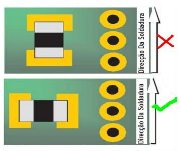
This way we also prevent the SMD's soldering to be affected and / or the component removed by selective soldering.
