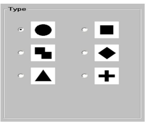
• Fidutial should not be equidistant in x, y to the board`s edge.
